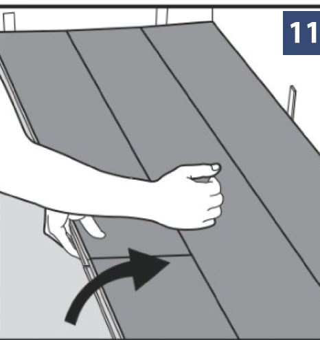
FIG 9 After 2-3 rows. Adjust the distance to the front wall by placing spacers.
